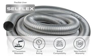
**SELFLEX**® is a double skin multi-fuel flexible chimney liner suitable for multi-fuel, gas, and oil-fired applications up to a maximum flue gas temperature of 600°C. CE marked to EN 1856-2. The SELFLEX® family range is suitable for the relining of masonry flues and used with wood, multi-fuel stoves and open fires and is available in three different specifications.
