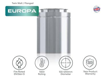
The **EUROPA®** product family consists of 3 flanged twin wall systems to suit a multitude of applications & all are constructed (as standard) from a 316L Stainless inner, 304 stainless outer & 25mm of insulation. All configurations are suitable for continuous flue gas temperatures up to 600C (T600) and positive pressure applications of up to 5000 Pa. The product family is for use with appliances ranging from coffee roasting machines to backup generators.
