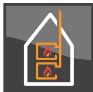
Decentralized multiple fireplaces connected to same chimney
